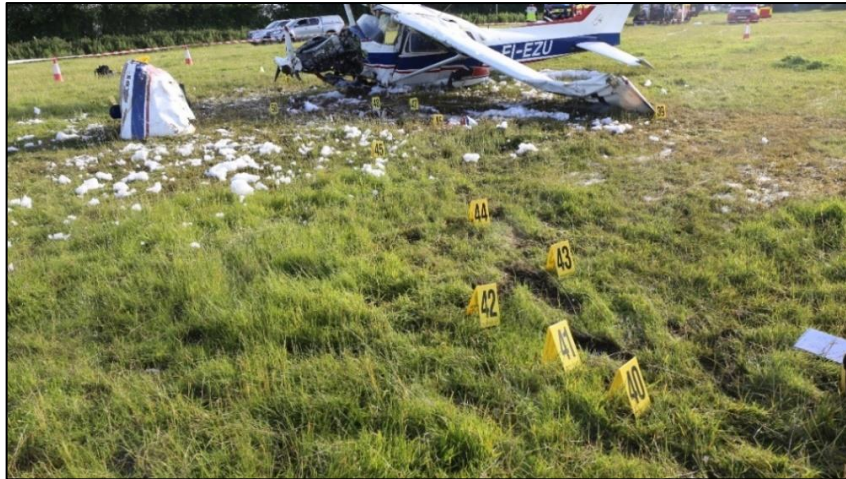
Photo No. 7: Ground damage outboard and forward of left wing
