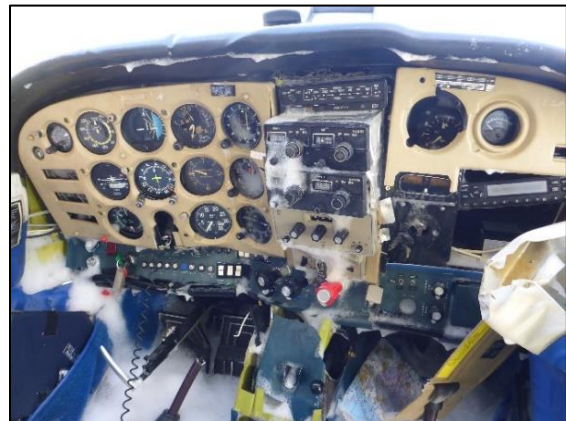
Photo No. 6: Damage to instrument panel and front foot wells
