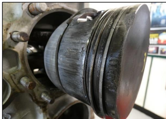
Photo No. 13: Damage to the No. 3 piston crown
