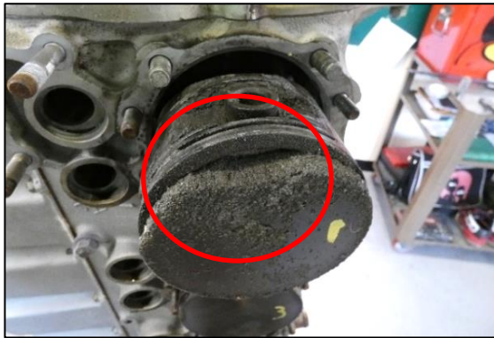
Photo No. 10: Damage to the No. 1 piston crown (ringed)
