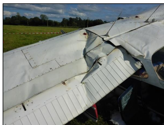
Photo No. 4: Creasing and bending on left wing's upper surface
