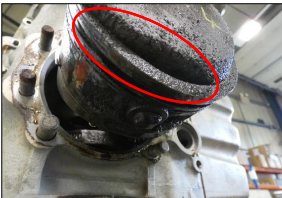
Photo No. 12: Damage to the No. 4 piston crown (ringed)
