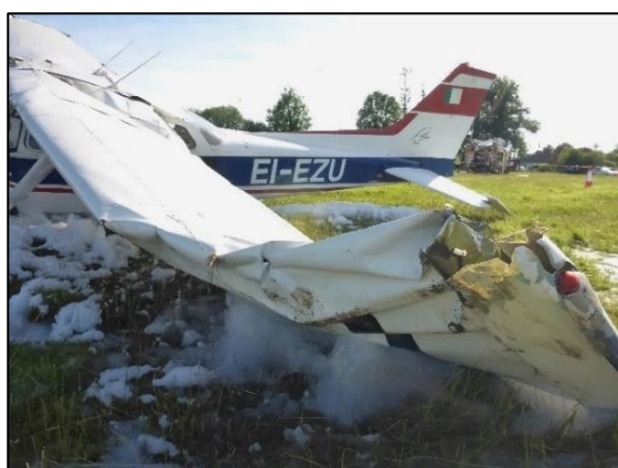
Photo No. 3: Damage to outer part of left wing
