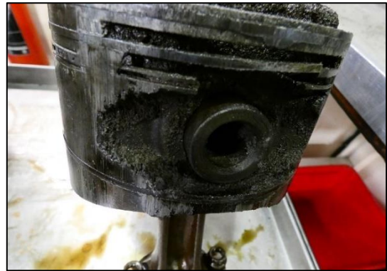
Photo No. 11: Damage to the No. 1 piston skirt and piston ring lands.
