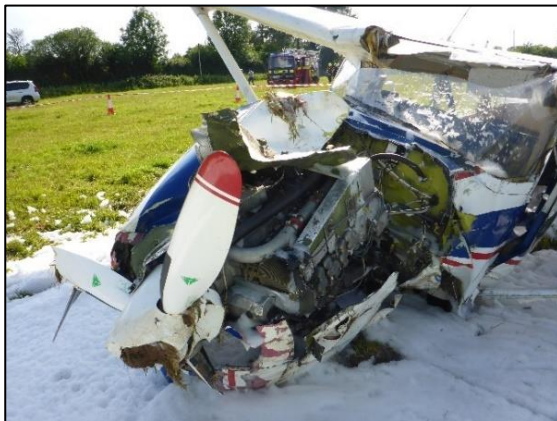
Photo No. 5: Damage to propeller blades and spinner
